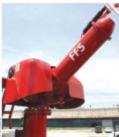
The tug's firefighting system has twin FFS monitors with a combined capacity of more than 10,000 gpm.
