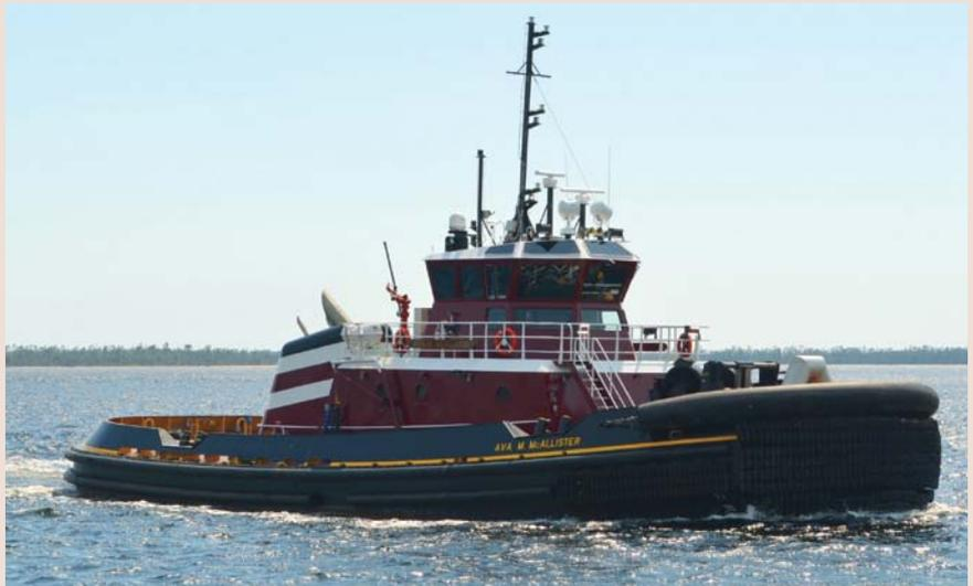
each rated at 1,500hp at 1,600 rev/min. The reduction gears are direct coupled Twin Disc Model MG-5600 with a 6.04:1 reduction. Electrical power is provided by two 99kW John Deere 4045AFM85 EPA Tier 3 generator sets.
