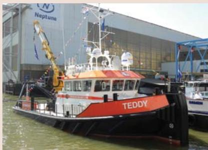
A Shoalbuster 2308 is the latest addition to the fleet of Dutch marine services company Herman Sr Tug and Workboat Company following its delivery in May. Named **Teddy** and built by **Damen Hardinxveld**, it is the second of its type and the 13th Damen vessel to be ordered by the family-owned operator based in Dordrecht.
