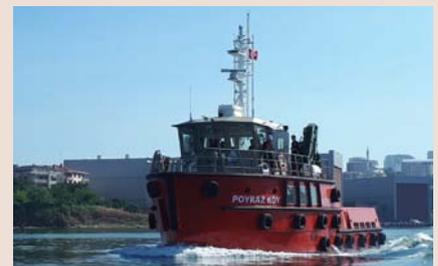
Propulsion is by twin fixed-pitch propellers driven by Volvo D13 engines each rated at 400kW for a top speed of around 11.5 knots depending on the outfit and loading. Nozzles can be fitted for better towing performance, but with reduced top speed.
