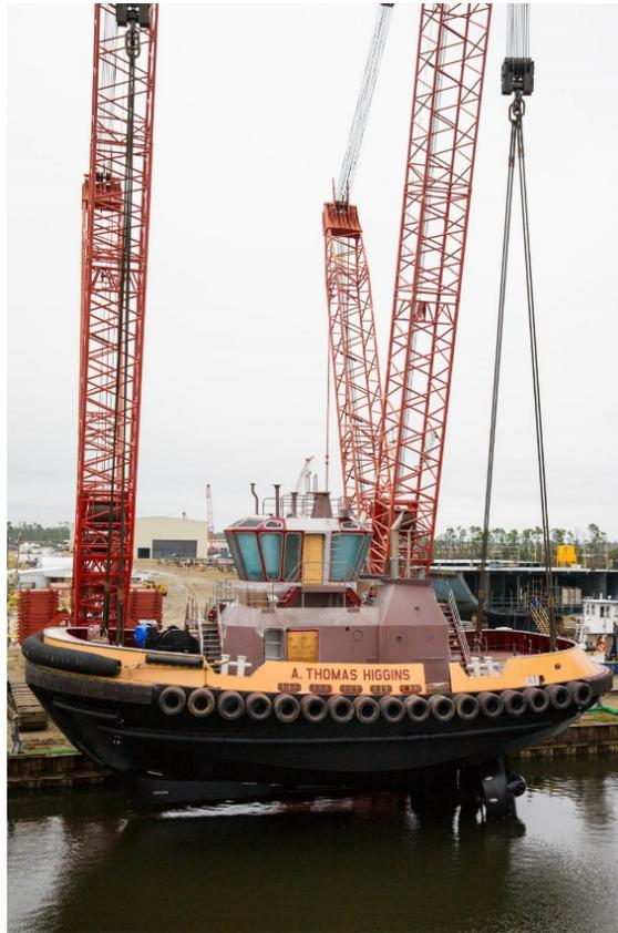
*Eastern's Twin Manitowoc Crawler Crane Tug Launch @ 380 Short Tons.*
