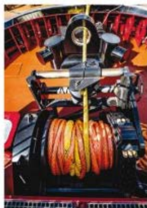
The Markay single-drum DEPCF-42 winch, right, is spooled with 400 feet of Samson Saturn-12 line. Below, C.D. White's 2,550-hp Cat engines are paired with Kongsberg/Rolls-Royce z-drives.
