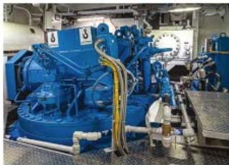
The Markay single-drum DEPCF-42 winch, right, is spooled with 400 feet of Samson Saturn-12 line. Below, C.D. White's 2,550-hp Cat engines are paired with Kongsberg/Rolls-Royce z-drives.
