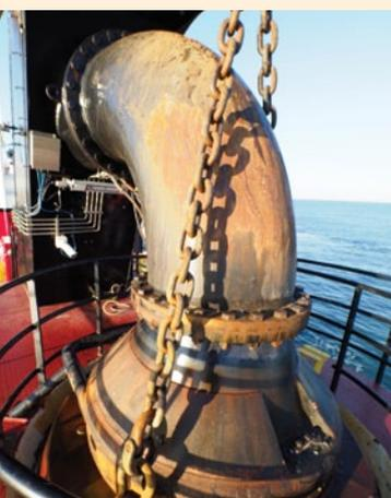
*Magdalen*, above, dredges the borrow area on the ocean floor 6.5 miles off Surf City, N.J. The vessel’s bow coupling, left, hydraulically locks the float hose to the discharge pipe system.
