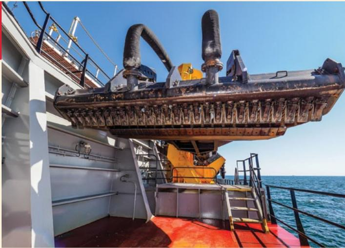
*Magdalen's* massive drag head stands ready to be deployed as the ship heads to the dredge site.
