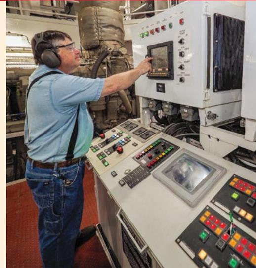
Chief engineer Scott Sirois, above, adjusts controls on the local operating console for the main engines. Below, *Magdalen* drag tender James Willis monitors the discharge of dredged sand to the beach.
